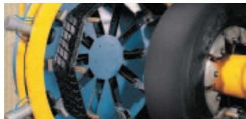
The spliceless UniCircle tread ring is slid over the buffed casing using special UniCircle equipment.
